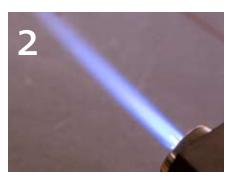
Adjust to a small oxydizing flame.
