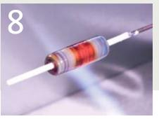
Re-introduce the bead at the top of the flame and slowly reheat until it starts to glow orange. Take it out of the flame and brown tones should bloom at this stage.
