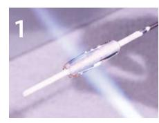
Start by winding Clear onto the mandrel in a barrel shape with a footprint of about 1.25"/32mm.
