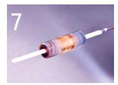
Take it out of the flame and gently marver the middle as it is cooling. Allow the glass to cool until the glow is gone. Carefully place the bead under the table to verify.
