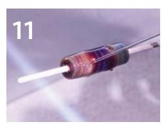
Repeat spot heating and twisting a total of three times on each side of the central dark purple band.
