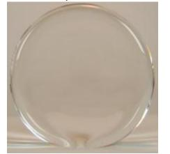
Zephyr is our clear glass that has been formulated to melt smoothly and easily in the torch; resist boiling and scumming; have a low reactivity with silver glasses; exhibit a low seed count and be fingerprint and dust free. Every pot of Zephyr is tested compatible with Effetre clear.
